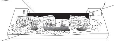
Figure 23. Install the Center, Left and Right Logs on the pegs.
